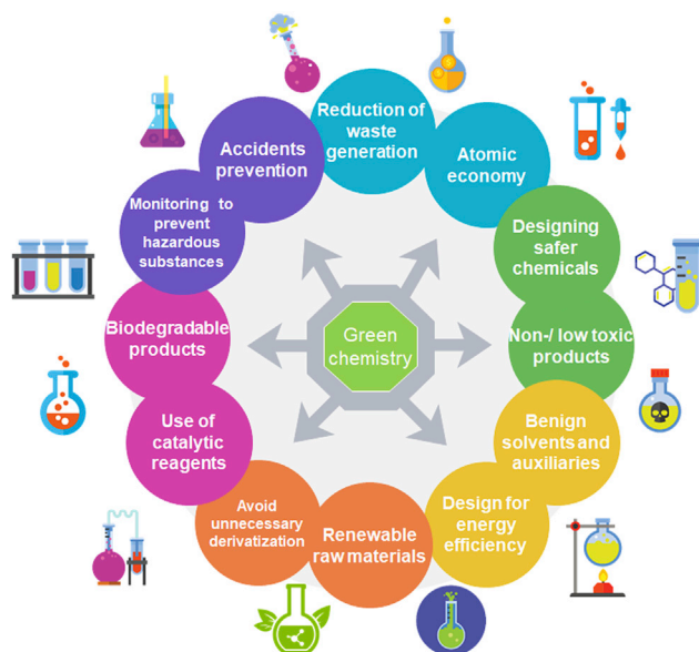
Figure 2. Twelve principles of Green Chemistry are based on the minimization of toxic solvents and non-generation of residues
